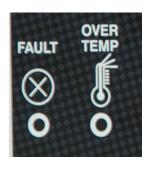
**FAULT** - **(Gas Only)** When this error is lit an ignition failure of the appliance has occurred. following the following steps:
